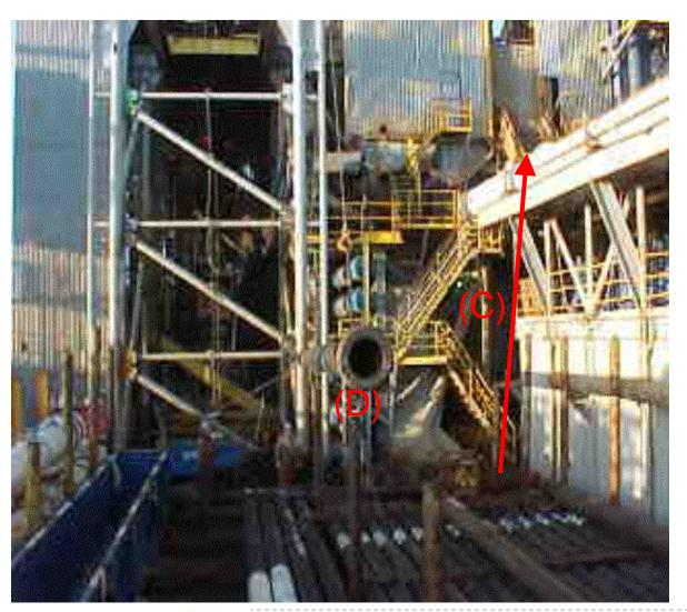
(C) Casing joint is lifted from the pipedeck to the catwalk area
