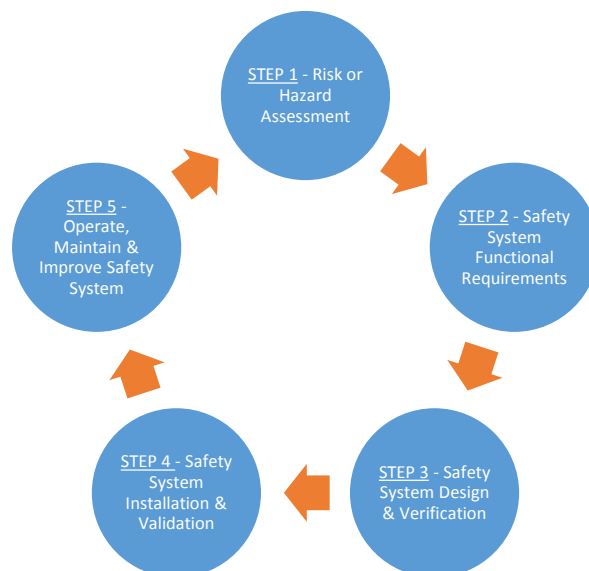
Figure 1 – Functional Safety Lifecycle Overview
